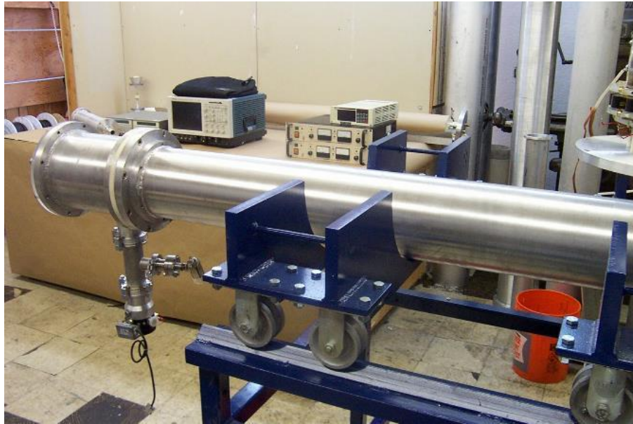
Figure 5 Example of the MG40-3C-2700PF Marx Generator with an attached X-ray diode
