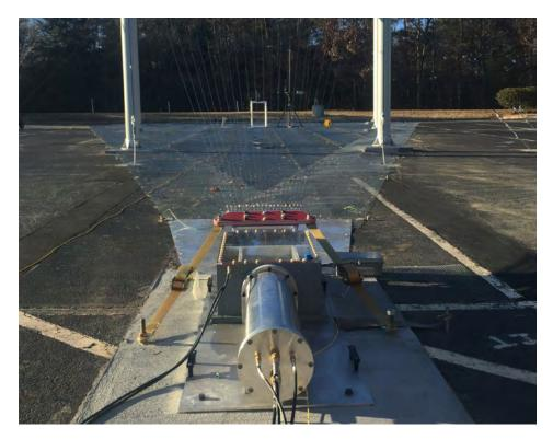
The APELC RS-105 test system utilizes APELC's compact Marx Generator technology to generate a pulse in accordance with MIL-STD-461G, test procedure RS-105. Test volume dimensions can accommodate a 2m × 4m × 4m in accordance with the MIL-STD.
