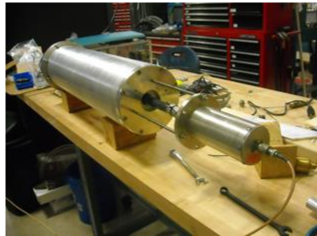
Figure 2. The stage-2 trigger generator being bench-tested for a ringdown test.
