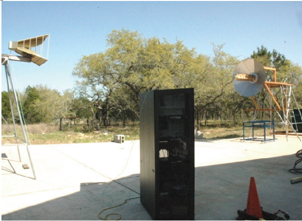
Figure 4. 400-MHz helical antenna VNA testing
