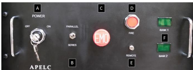
Fig. 3. HCADS Power and Control Panel (Front): (A) Power key-switch (controls), (B) Parallel/Series toggle switch, (C) Emergency-Off Button, (D) Fire Button (Momentary push), (E) Fiber optic remote input, (F) Bank 1 and 2 charge voltage LED indicators.
