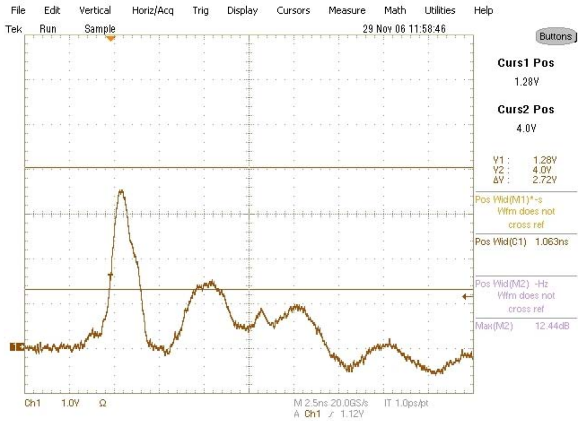
Figure 7. An initial time domain measurement made from the APELC linear half TEM horn antenna when excited by a 60 kV pulse.
