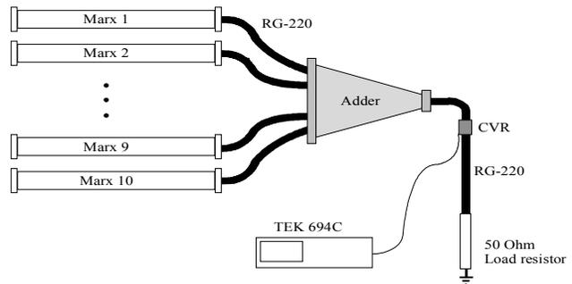
Figure 5. Experimental arrangement.
