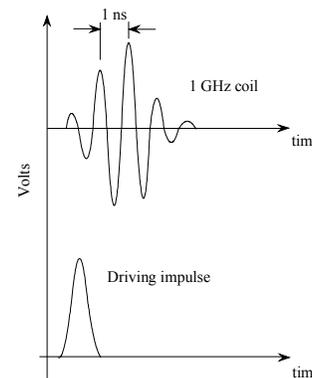
Figure 3. Illustration of a single Marx driving a 1 GHz coil antenna.
