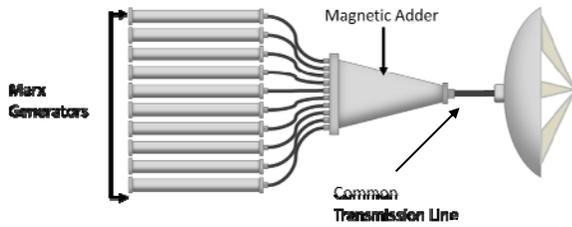
Figure 1. An illustration of the Gatling Marx generator system.
