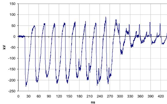
Figure 7. Output waveform of the nine-pulse Gatling system.
