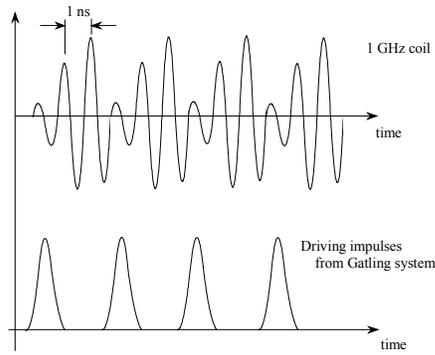
Figure 4. Illustration of the Gatling Marx generator system driving a 1 GHz antenna.
