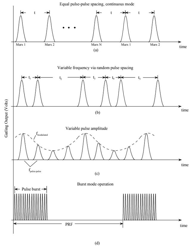
Figure 2. An Illustration of functionality with the Gatling Marx system. (a) equal pulse-to-pulse separation, (b) random pulse-to-pulse separation, (c) modulation of pulse voltage levels, and (d) burst mode operation.
