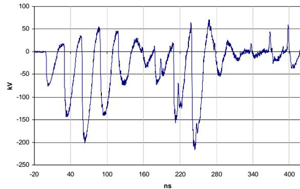
Figure 9. A simulated Gaussian wave shape produced by the Gatling system.
