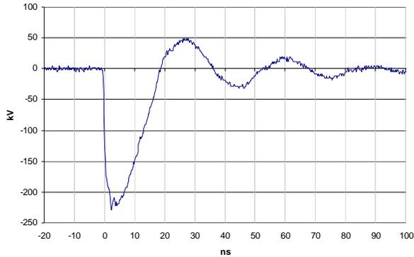
Figure 6. Resulting waveform of a single pulse through the magnetic adder.
