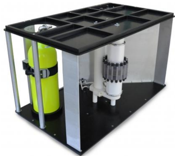
Figure 3. Footlocker skeleton showing the Marx generator mounted behind the antenna inside the corner reflector.
