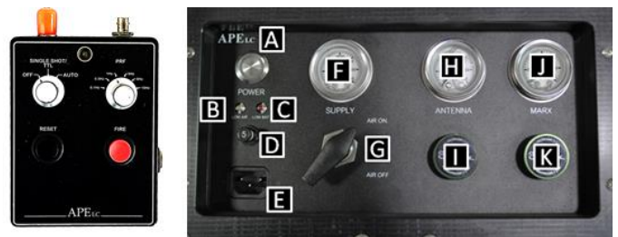
Figure 4. (left) handheld fiber-optic controller, (right) Interface Panel: (A) Power switch, (B) low air light, (C) low battery light, (D) push/pull circuit breaker, (E) charge port, (F) cylinder pressure gauge, (G) gas shut-off valve, (H) antenna pressure gauge, (I) antenna pressure adjustment, (J) Marx pressure gauge, (K) Marx pressure adjustment.
