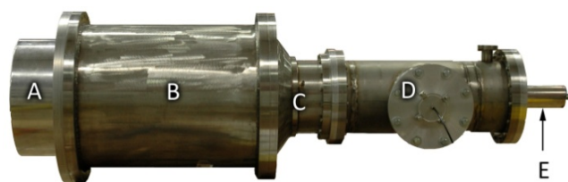
Figure 1. Main components of the APELC Marx Generator system: (A) power/control module, (B) Marx generator circuit, (C) diagnostic/transition flange, (D) load module, and (E) CVR.
