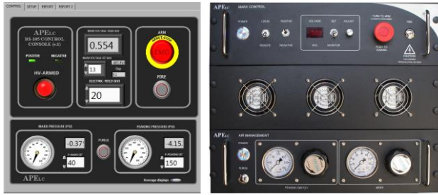
Figure 11. Remote control software (left) and local controls (right)
