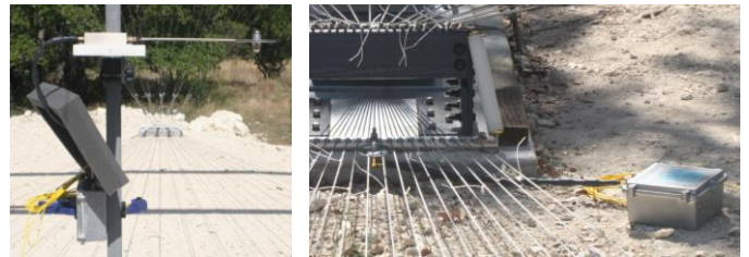
Figure 10. Prodyn AD-55 free-field D-dot sensor (left) and Prodyn AD-110 ground-plane D-dot sensor (right)
