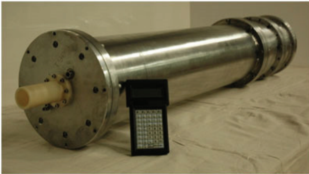
Figure 2. Marx Generator with Attached Capacitor Charger
