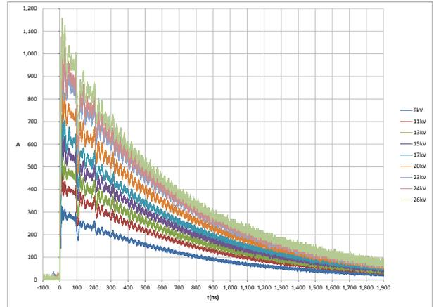
**Figure 2.** Marx generator output into a short circuit (charge voltage varied from 8kV to 30kV)
