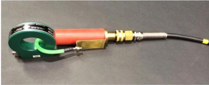
**Figure 4.** Direct-connect fixture (shown with Pearson current transformer)
