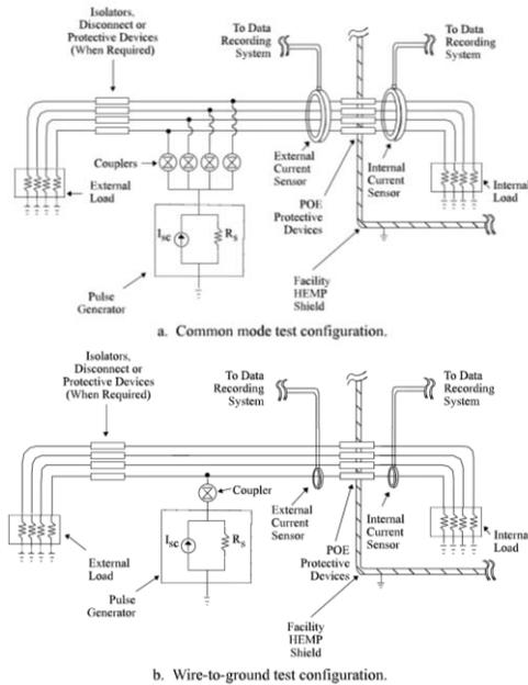
**Figure 1.** Pulsed current injection test configurations
