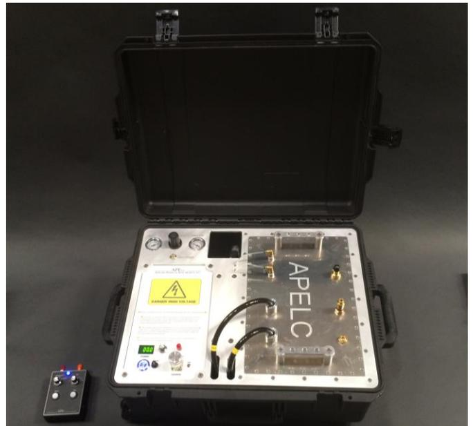
**Figure 3.** Two-stage Marx generator PCI system
