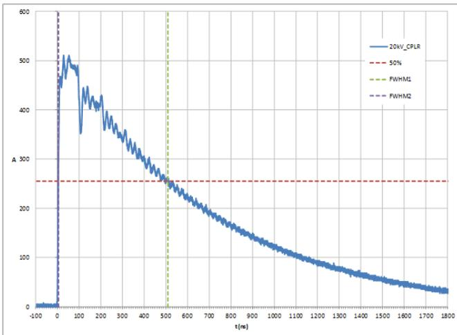
**Figure 6.** 500 Amp waveform using the inductive coupler
