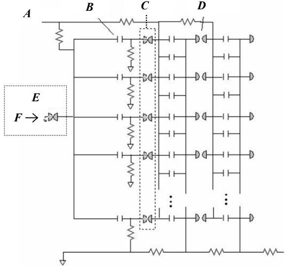
**Figure 3.** The trigger scheme of the APELC Marx topology. High voltage in (**A**), trigger capacitor (**B**), Parallel (stage) trigger gaps (**C**), stage capacitor (**D**), Main trigger gap (**E**), trigger in (**F**).
