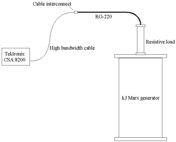
**Figure 7.** A TDR measurement made on the Marx load.
