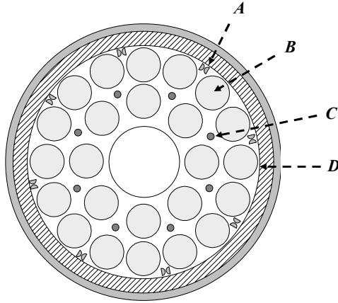
**Figure 2.** The APELC Marx generator MG20-24C-2000PF stage topology. Parallel spark gaps (**A**), door knob capacitors (**B**), support rod (**C**), and epoxy liner (**D**).
