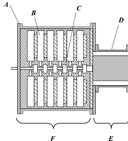
**Figure 1.** A traditional Marx design for HPM systems. Marx generator (**A**), Maxwell capacitor (**B**), Maxwell spark gap switches (**C**), PFL (**D**), Energy related to pulse length (**E**), 10x energy stored in PFL (**F**).
