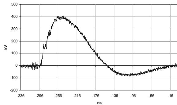
**Figure 10.** Output waveform with a  $40\text{ kV}$  charge.
