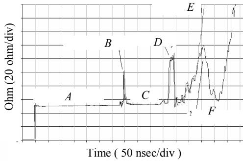
**Figure 8.** TDR measurement of Marx generator. Solid line. High bandwidth cable (*A*), cable interconnect (*B*), RG 220 (*C*), CVR cavity (*D*), Load removed (*E*), Marx load in place (*F*)
