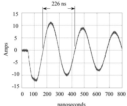
**Figure 5.** The CVR-measured ring-down. Ring down period  $\tau=226$  nsec..
