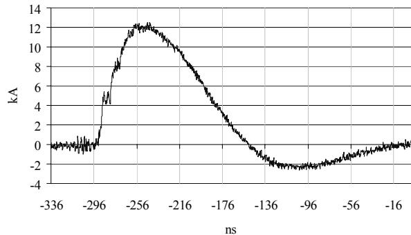
**Figure 6.** Output waveform with a 20 kV charge.
