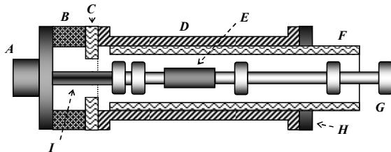
**Figure 4.** Load design and diagnostic tools for the APELC Marx generator MG20-24C-2000PF. T&M Research CVR (**A**), extension collar (**B**), acrylic insulator (**C**), aluminum housing (**D**), Kanthal resistor (**E**), acrylic liner (**F**), aluminum feed (**G**), capacitive voltage probe collar (**H**), internal conductor (**I**)
