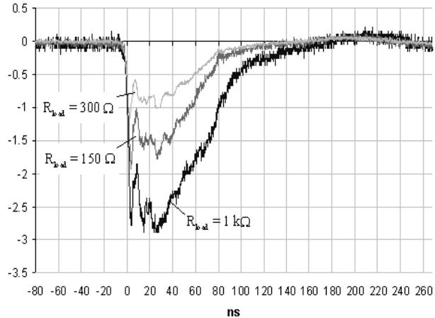
**Figure 9.** Output waveforms with various load resistors.
