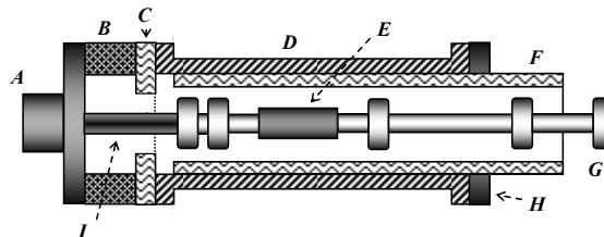
**Figure 4.** Load design and diagnostic tools for the APELC Marx generator MG15-3C-940PF:
