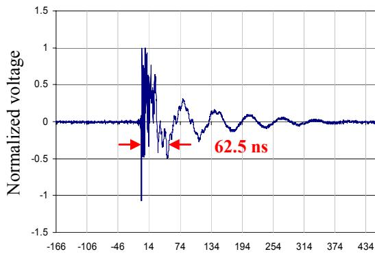
**Figure 5.** The Pearson-measured ring-down.
