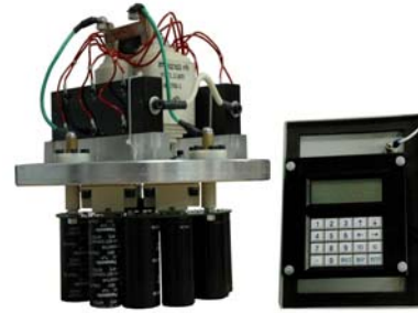
Figure 3. Photograph of the Rapid Capacitor Charger and controller.
