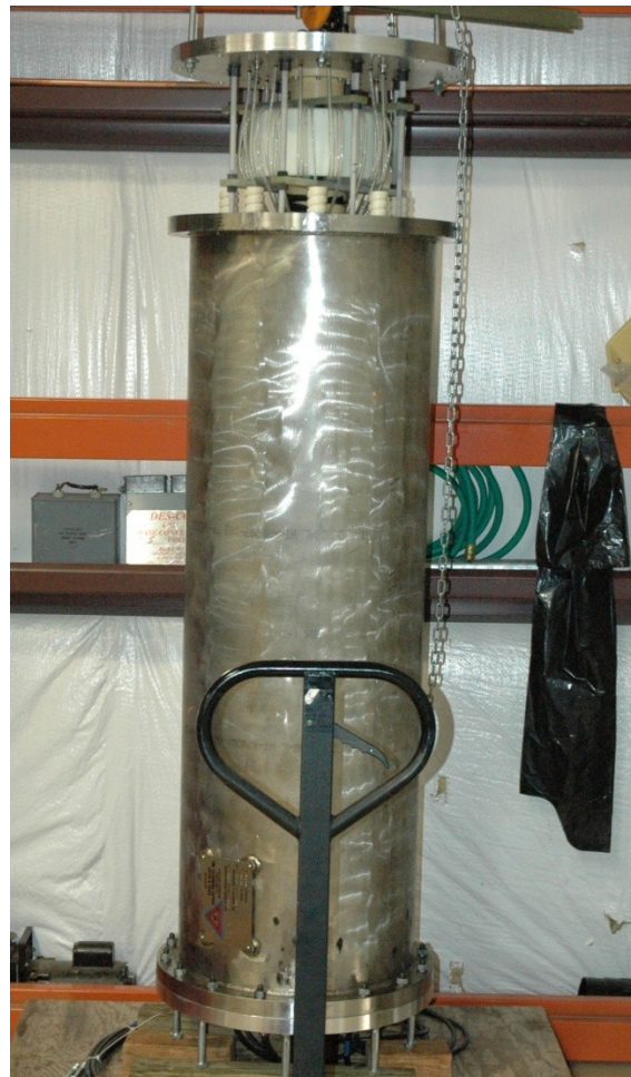
Figure 1. APELC EBU erected-PFN pulse generator shown being installed in pressure housing.
