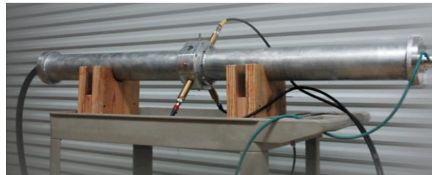
Figure 6. Experimental prototype dual polarity Marx generator source.
